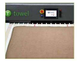
Pieces are put on the intake conveyor belt. This conveyor belt starts running once the piece is detected or after manual activation with a
