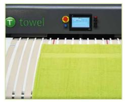
The **T.towel** is provided with a special feature to fold pieces that need extra corrections before being folded, like fitted sheets. After placing the sheet on the feeding table and pushing the button, the piece runs inside the machine and makes an automatic stop for correcting the tail end of the piece. Then, the operator pushes the button a second time so
