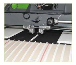
In case two folders are put next to each other, each can have its own final delivery belt. Alternatively, both machines can be interconnected in master/slave configuration. Piles from both machines are put on one final delivery belt, allowing automatic direction of all piles towards a central conveyor belt leading to a packing/ wrapping machine.
